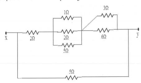
3. a)Find the current through each resistor of the circuit shown in below figure.
